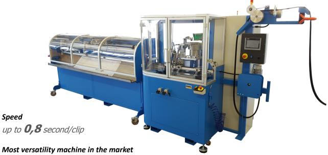
You want to run another program with different clips? By changing quides, profile-specific puller/clamps, VIBRATOR BOWL and the recipes, our machine allows you to run an almost infinite number of cross sections and CLIPS.
