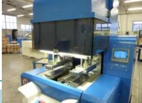
The SJ-PE MAXI multipurpose jointing system is the latest technology for the production of butt and corner joints in profiles made of (reinforced or non-reinforced) rubber, thermoplastic materials and PVC.
